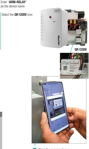
Place the camera of your Smartphone in front of the QR CODE to acquire, automatically, the ID of the relay device
