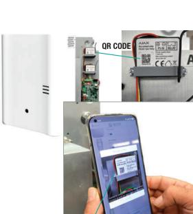
Place the camera of your Smartphone in front of the QR CODE to acquire, automatically, the ID of the relay device
