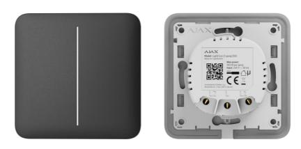
A single LightSwitch consists of two elements: a **LightCore** relay and a **SoloButton** touch-sensitive panel.
