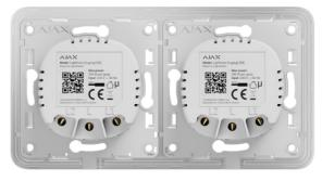
A combined switch consists of several **LightCore** relays and touch-sensitive panels installed in one frame with the appropriate number of seats.
