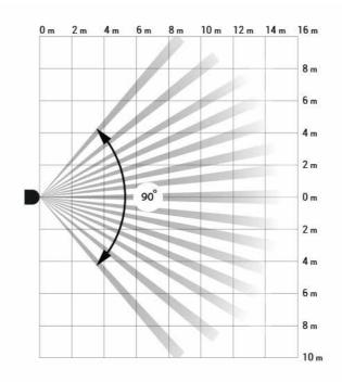
Make sure that no obstacles block the view of the detector. Note that MotionCam Outdoor does not detect movement behind the glass. Therefore, do not install the detector in locations where an open window or door can obstruct its view. When installing, also consider the width of the detection zone. Incorrect detector placement can lead to false alarms.
