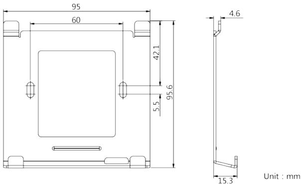
Figure 5-1 Wall Mounting Plate
