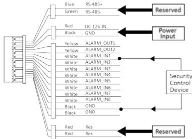
**Figure 4-1 Wiring Description (Alarm Input Device)**
