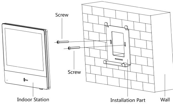
**Figure 5-2 Installing the Plate**
