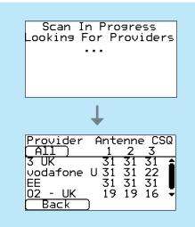
For a reliable 2/3/4G connection it is recommended that for the chosen network (SIM card) used there should be at least two base stations with signal strength (CSQ) of 10 or more.
