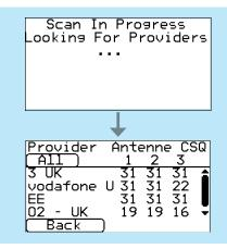
For a reliable 2/3/4G connection it is recommended that for the chosen network (SIM card) used there should be at least two base stations with signal strength (CSO) of 10 or more.
