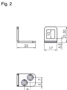
Prepare door frame so that STEP 36 fits in it, for measurement use template drawing.
